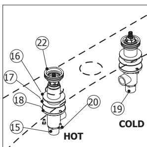
**C.** Do the same on cold valve(19). Make sure your valve outlets are directed toward the spout.
