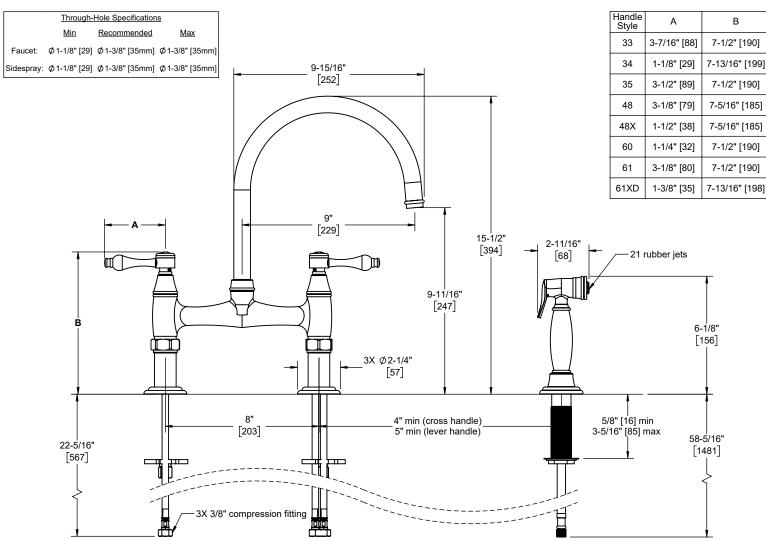
Dimensions are inches, rounded to 1/16" [Dimensions in brackets are mm, rounded to 1mm]
