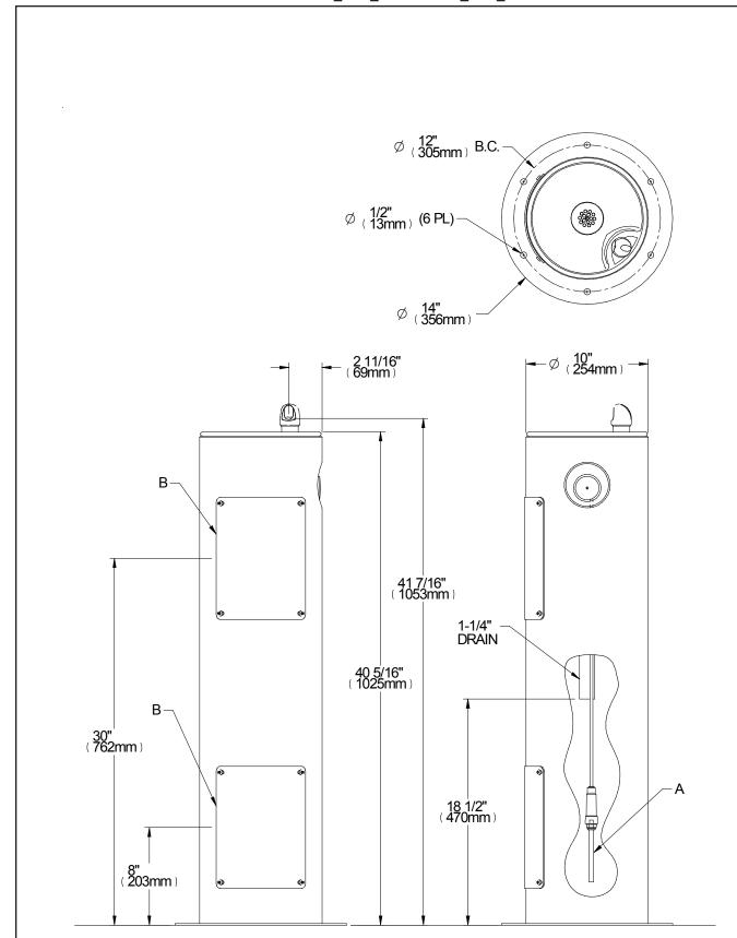
LEGEND A = 3/8" O.D. UNPLATED COPPER TUBE CONNECT - SHUT OFF VALVE BY OTHERS  $B = ACCESS\ PANEL\ (8"\ X\ 10")$
