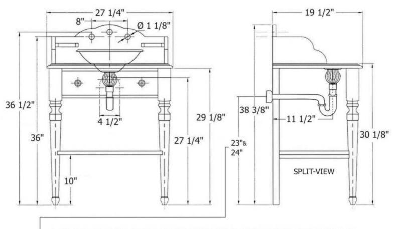
\* ALL DRAIN MEASUREMENTS ARE USING THE 2124, 3013 or 3014 DRAIN ASSEMBLY
