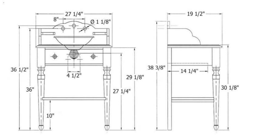
ALL DRAIN MEASUREMENTS ARE USING THE 2120, 2121 & 2122 DRAIN ASSEMBLY
