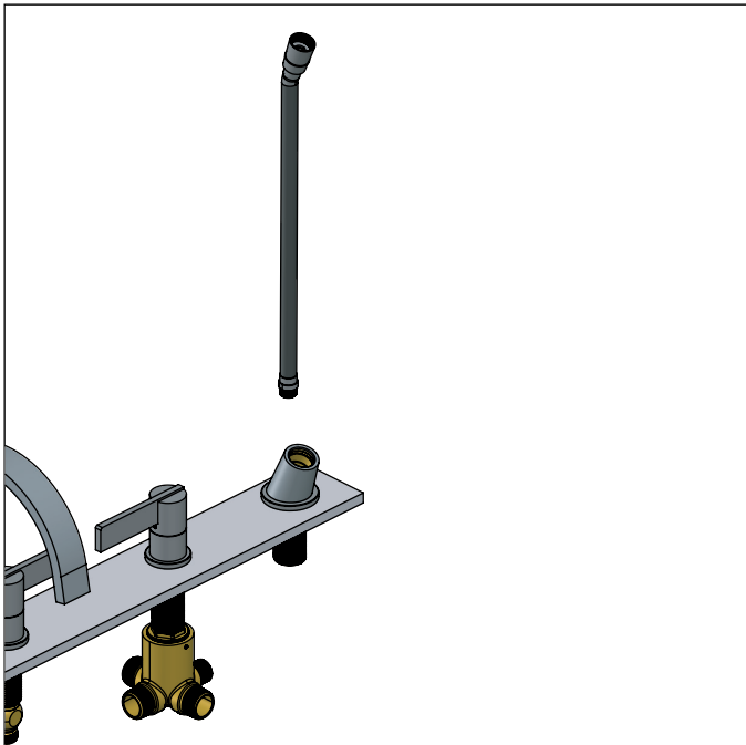
Drop hose down through deck hole
