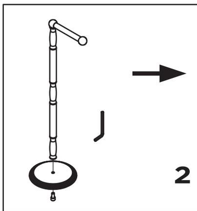
Align the tissue holder to the mounting holes on the bottom part, and use the Allen key to screw through from the back of the bottom and tighten it.
