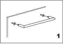
Install the vertical handle (bolt) through the glass holes, make sure the rubber gaskets are between handle&glass.
