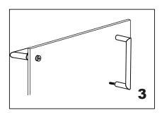
Install the horizontal handle (bolt) through the glass, make sure the set screws holes in the bottom.
