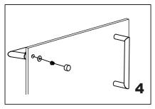
Screw in the bracket onto the bolt,fix the backing (end cap) onto the bracket
