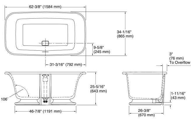
**PRODUCT INFORMATION** Fixture\*: Top Area Basin Area Weight 60-9/16" (1539mm) x 44-5/16" (1126 mm) x **Bathing Well** 474 lbs (215 kg) 32-5/16" (820mm) 24-3/16" (614 mm) Water Depth Capacity To Overflow 16-1/2" (419 mm) 78.3 gal (296.2 l) \*Approximate measurements for comparison only.
