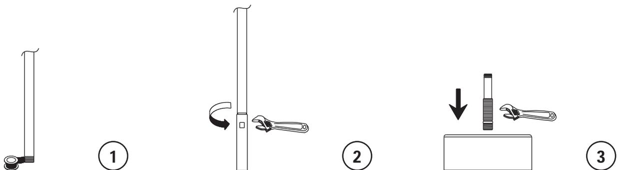
**1** Apply pipe tape to the threads of the water pipe.
