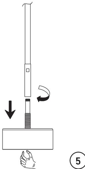
**5** After the construction and decoration of the ceiling is finished, remove the internal pipe with the plastic drum by hand.
