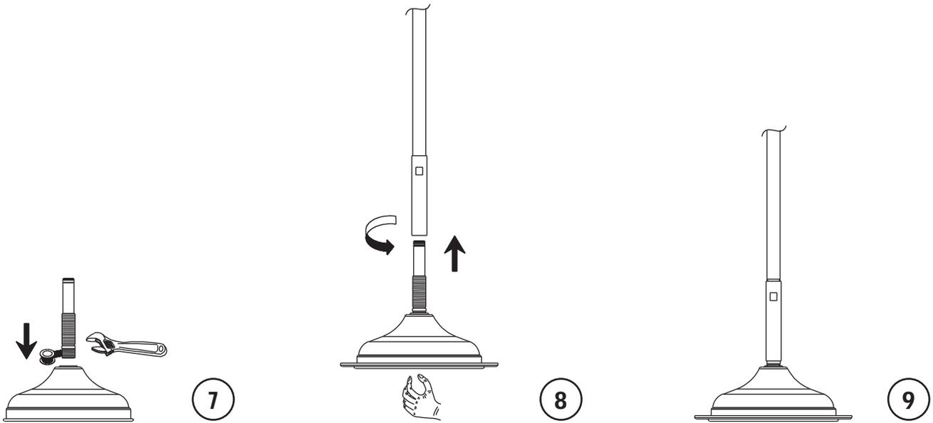
**7** Apply pipe tape on the threads of the internal pipe. Then tighten the internal pipe to the showerhead with wrench.
