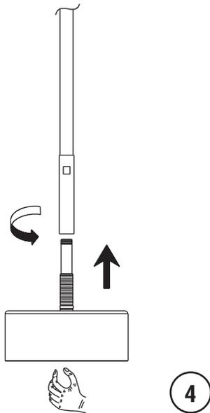
**4** Install the assembled internal pipe and plastic drum to the connecting tube, then adjust to an appropriate position (the degree of adjustability is 45mm).
