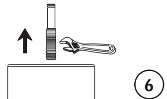
**6** Disconnect the internal pipe from the plastic drum by wrench.
