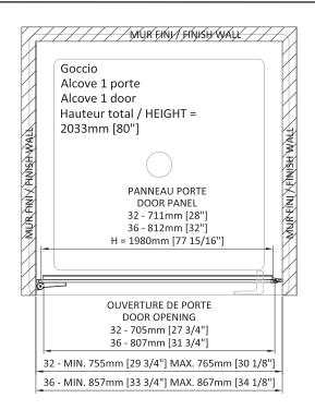
Door 32" Gauche : DGC3200ASTG21 Door 32" Droite : DGC3200ASTH21 Box #1 80 1/8" x 29 3/8" x 3 2035mm x 745mm x 75mm 75 lb (34 kg)
